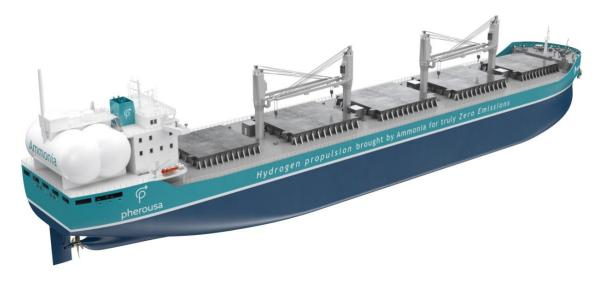
Deltamarin, a renowned ship design and engineering company with a strong focus on alternative fuels and decarbonization in deep-sea shipping, has developed an innovative long endurance ammonia fueled Ultramax bulk carrier concept together with PGT.
